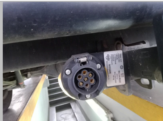
Trailer plug cover missing
