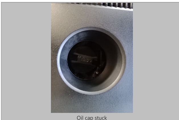
Oil cap stuck
